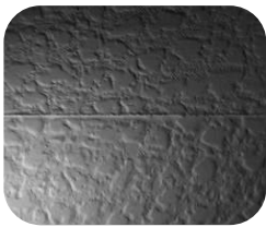
Parting line and texturing of a steering wheel
