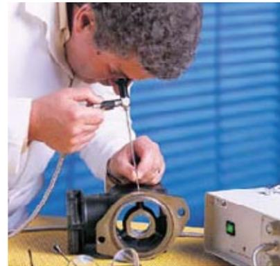
Inspecting air-brake compressor after machining
