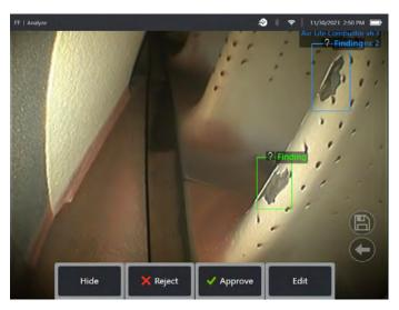
Initiate 'Freeze Frame' to activate Aiir Lite - Combustor analytic.
