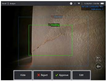
Once the image is saved and then subsequently recalled, only the accepted bounding box(es) will be immediately visible. This image shows the one bounding box that was 'accepted'. All others remain present but 'hidden' within the file.
